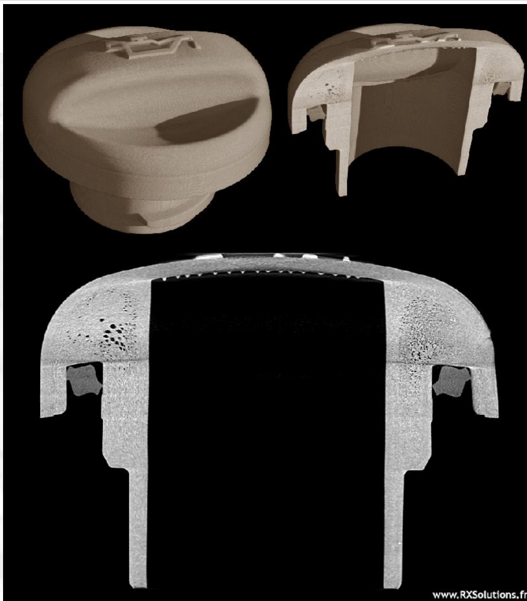
Porosities in plastic oil shutter
